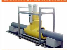
Gamma spectrometer SEG-001 "AKP-S" "KERN" is designed for express analysis of full-length core samples to determine the natural gamma-ray emitting radionuclides <sup>226</sup>Ra, <sup>232</sup>Th, <sup>40</sup>K and artificial <sup>137</sup>Cs and other in rock samples. Binding data logging to the core depth.
